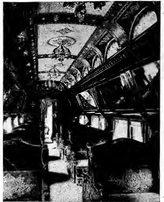
Fig. 126. INTERIOR OF SLEEPING CAR AMERICA. Exhibited at World's Columbian Exposition, 1893, by Pullman's Palace Car Company. Vaulted Ceiling, Oval Deck-Windows, Disappearing Curtain Rods and Electric Lights. (Plan is shown in Fig. 186.)
